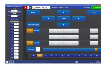
Nicknumbers are stored locally and will be remembered each time the app is opened. To reset a nicknumber, tap the button next to the camera's nicknumber display.
